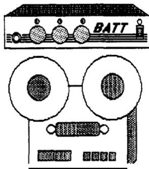
**RACK MOUNTING / BASS MASTER STAGEBOARD:** The BATT can be used as a stand-alone preamp or as an extension to an existing system. Hughes & Kettner offer special single and twin adaptors to facilitate 19" rack mounting. A Sound Machines STAGEBOARD is optionally available for easy on-stage switching of two units (Unit1 / Unit 2 / Bypass ).
